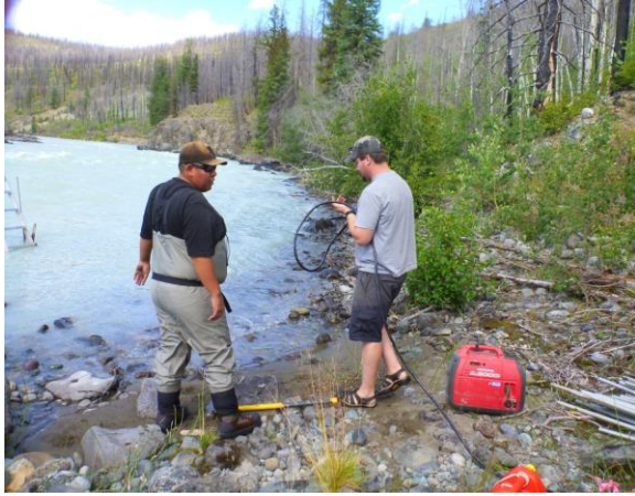
3) Laying out the DIDSON cable and setting the DIDSON view.
